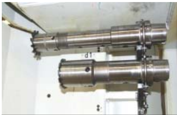
Reamers stay in the tool magazine and are used in all materials with the same tight tolerances, no adjustment.
