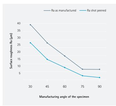
The surface quality was characterized by optical measurement method from down-facing surfaces according to internal procedure. The 90 degree angle corresponds to vertical surface.
