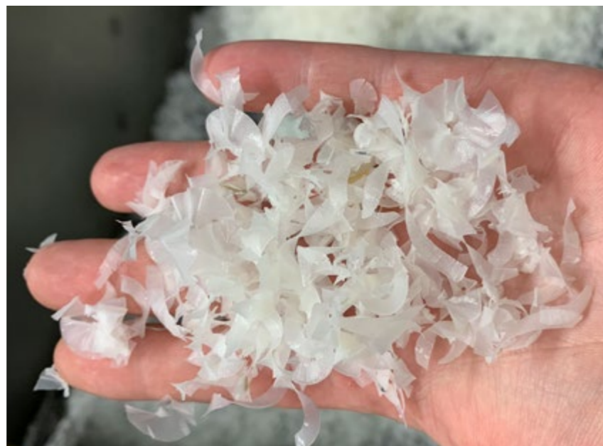
Chip formation during reaming
