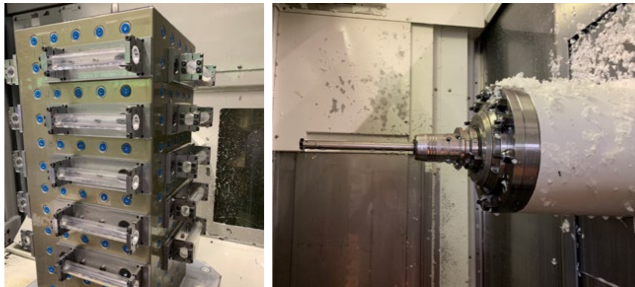
20 parts are clamped per tower. This results in a time saving of 189 minutes per tower!
