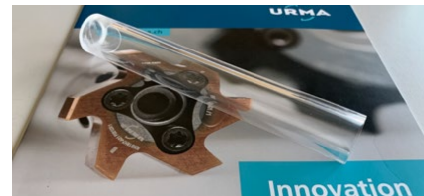
Finished reamed component - Ra 0.12 / Rz 1.05
