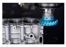
Thanks to the high tool rigidity of the MX diamond, both finishing and roughing cuts can be made with the same cutting edge. Source URMA AG
