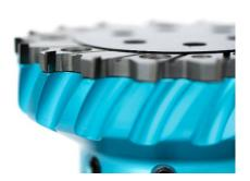
The teeth of the solid carbide cutting edge body are fitted with up to 20 PCD tips and are ideally suited for machining lightweight materials. Source URMA AG
