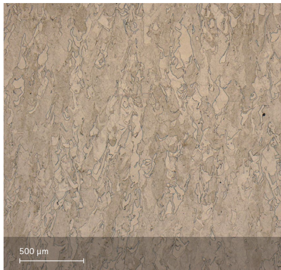
Microstructure solution annealed Etched with etchant Kallings 2
