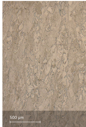
Microstructure solution annealed Etched with etchant Kallings 2
