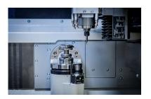
The microone micro machining centre is perfect for the production of movement and case components. In addition to the watchmaking industry, applications in medical technology rely on the machining of micro-components.
