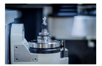
The ZORN CNC machine for precision micro parts is available with 3-axis or 5-axis simultaneous machining, and can also be customised.
